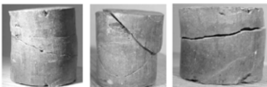
Figure 5-14: Macroscopic observations of cracks on boom clay samples under desaturation
