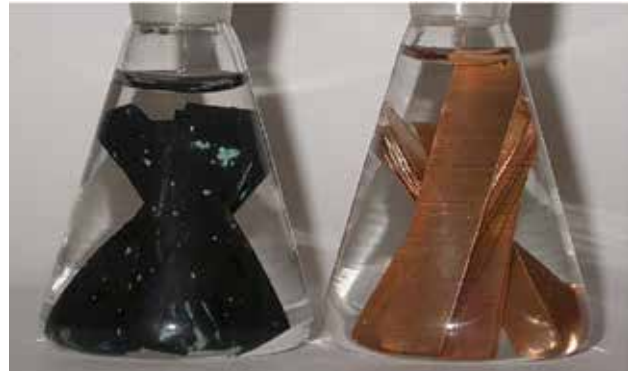
Appearance of copper after 15 years of exposure in distilled water at room temperature. Hydrogen from corrosion can escape from the left container but not from the container to the right. The water volume was equal in the flasks in beginning of the exposure.
