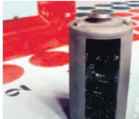
Figure 2 – Vitrified high-level metallic waste container
